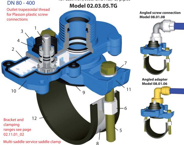
One bonnet including gasket for the dimensions DN 80 - 400. Stainless steel retaining bracket with large clamping range made of Band 60 x 1.5 mm for GGG / ST Band 90 x 1.5 mm for AC / FC
